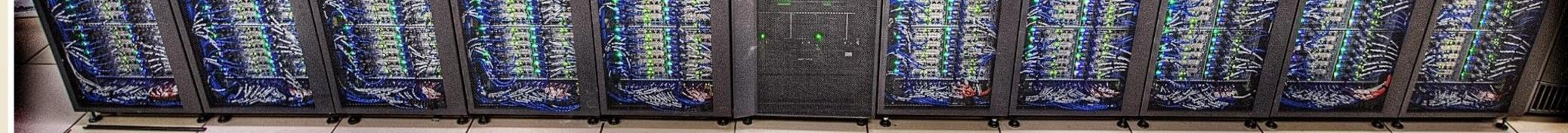
A 17,500-core system, with 845 20-core nodes equipped with the INTEL 10-core 2.5GHz lvyBridge processor. The other 15 nodes are 1TB and 2TB memory, 4-processor SMPs configured with the INTEL 10-core 2.7GHz Westmere processor. 30 nodes have 2 GPUs each and 9 have 2 Phi coprocessors. The interconnecting fabric is based on the Mellanox SX6536 IB core switch (the middle rack in the graphic above).
