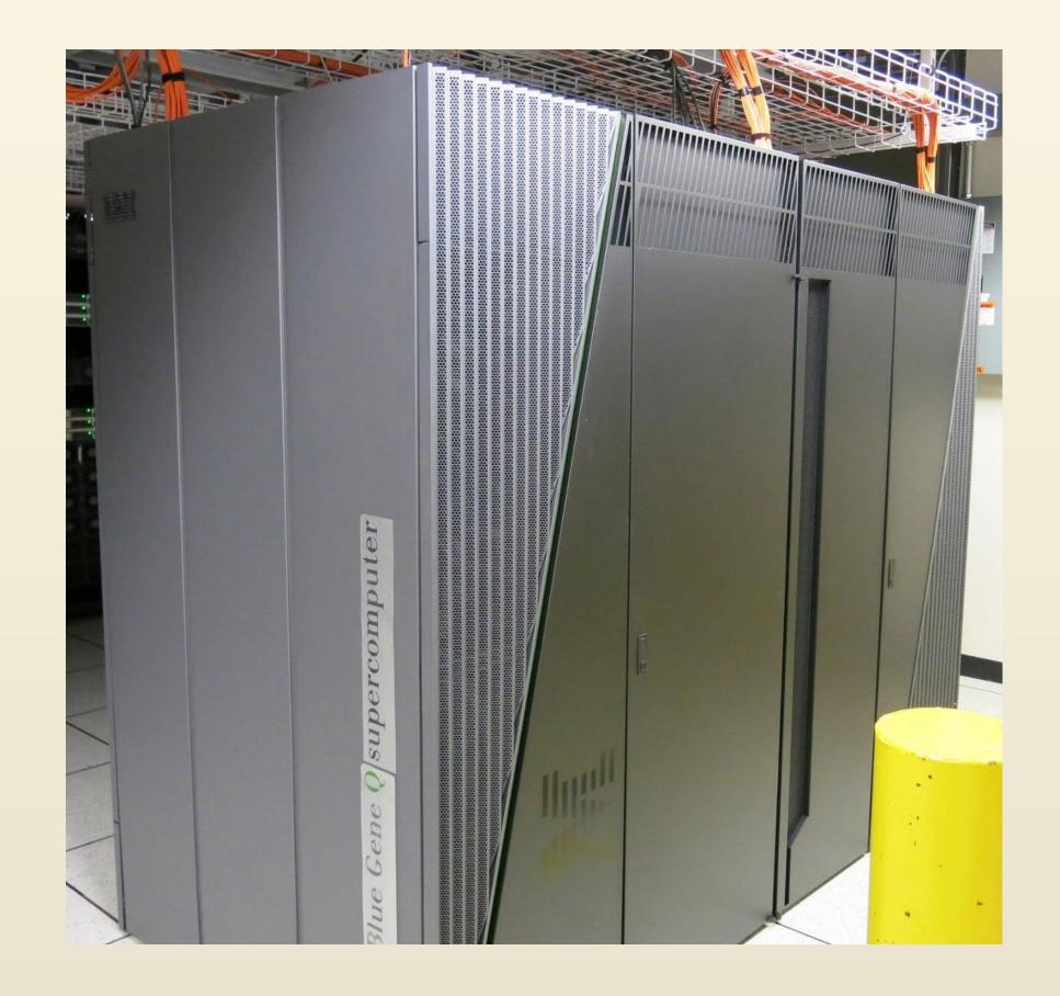
32768-core, 419 TFLOPS, Massively Parallel, interconnected in **5D Torus topology**
