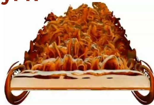
Flow past airfoil for Martian helicopters [2]
