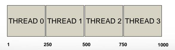
Although the OpenMP standard does not specify how a loop should be partitioned most compilers split the loop in N/p (N #iterations, p #threads) chunks by default.
