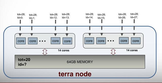
All threads try to access the same variable (possibly at the same time). This can lead to a race condition. Different runs of same program might give different results because of these race conditions
