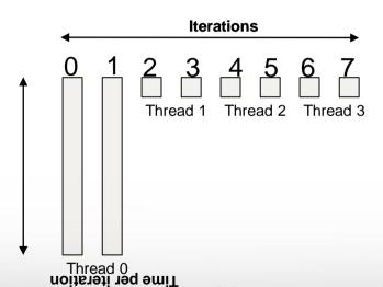
This is called load imbalance. In this case threads 2,3, and 4 will be waiting very long for thread 1 to finish
