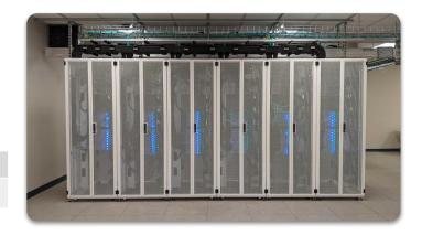
FASTER (Fostering Accelerated Sciences Transformation Education and Research) is a 180-node Intel cluster from Dell with an InfiniBand HDR-100 interconnect and Liqid PCIe Gen4 for composing the GPUs. Nvidia A100, A10, A30, A40 and T4 GPUs are available. The 180 nodes are based on the Intel Ice Lake processor.
